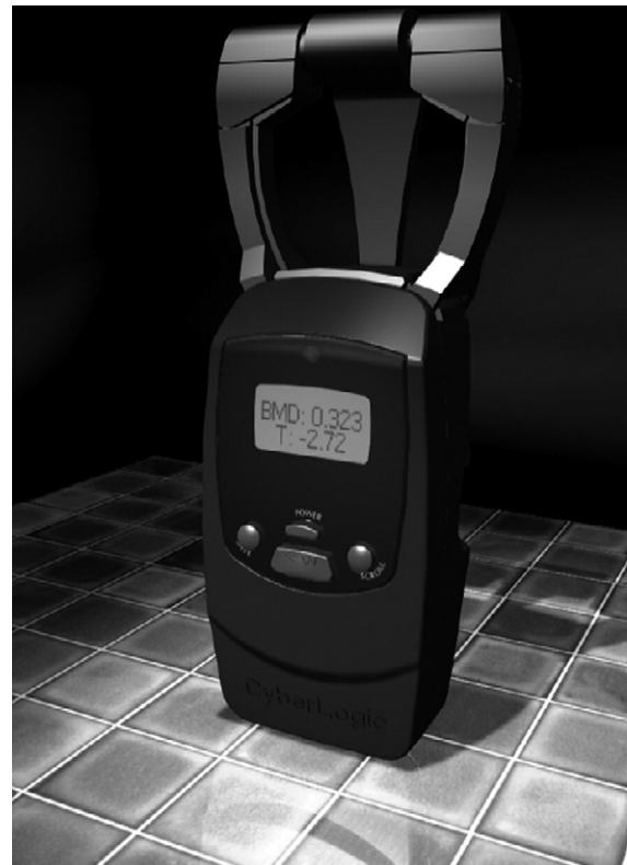
Fig. 4. Computer rendering of the QRT 2000 ultrasound bone assessment device. The overall height is about 23 cm, and the distance between the transducers as shown is 3.8 cm.
